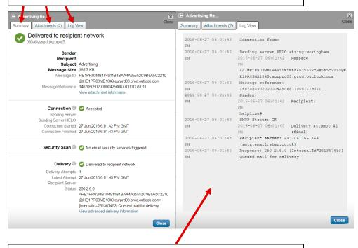
The log view provides a copy of the delivery log for a message. From this extract of the SMTP logs, it is possible to see where delivery was attempted and any errors that occurred during the attempt.
